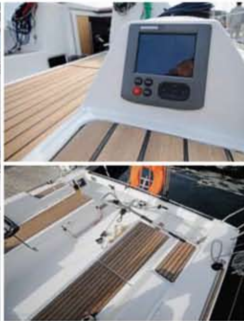
The cockpit (above) is huge, thanks to fat stern sections. No need for a binnacle with coaming ends housing electronic displays (top). Transom beam carries the traveller (left).
