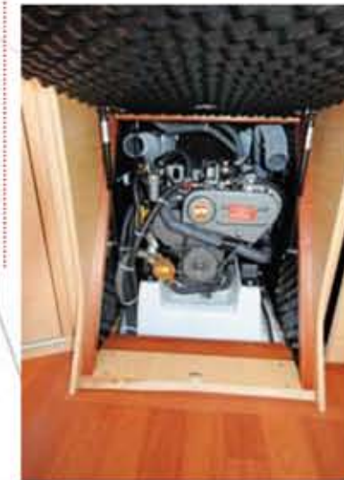
Extensive soundproofing lines the enginebox (above) for the 20hp Yanmar diesel.
